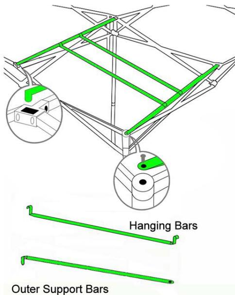
For each Outer Support Pole insert the crook end into the central slot.
