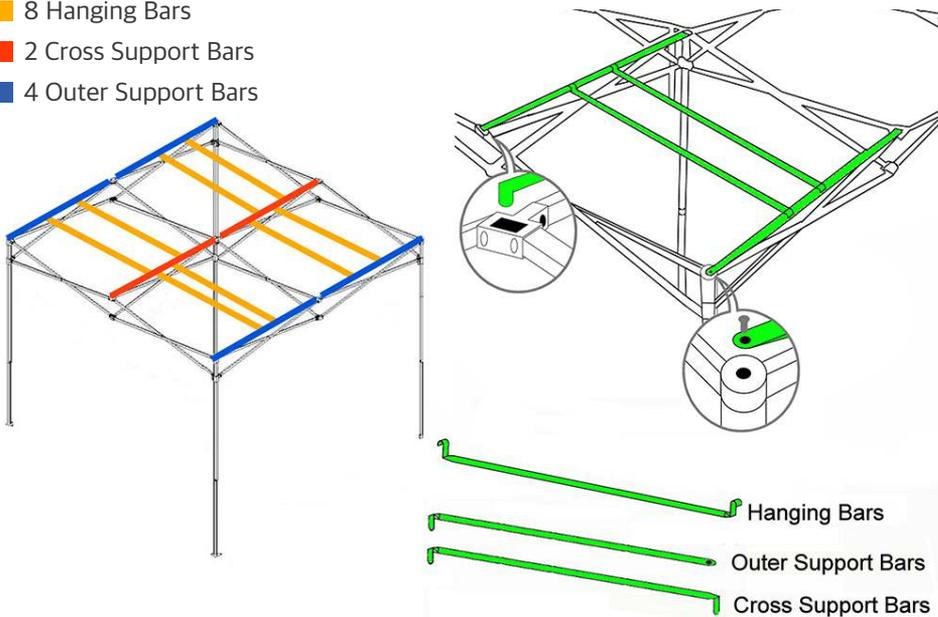
For each Outer Support Pole insert the crook end into the central slot.
