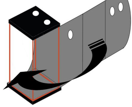
Insert the spill tray and secure with velcro ties.
