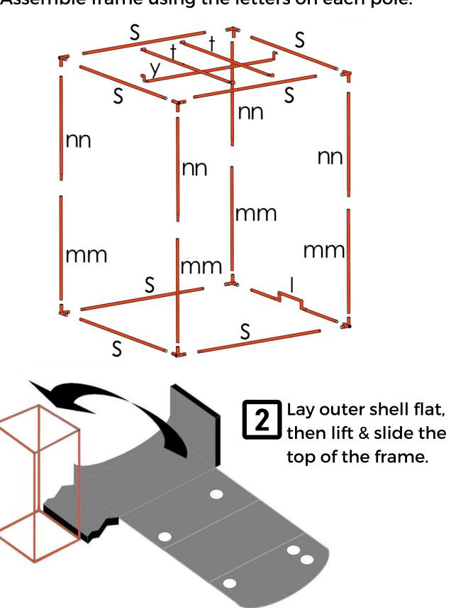
Slide the base (floor) of the outer shell under the frame.
